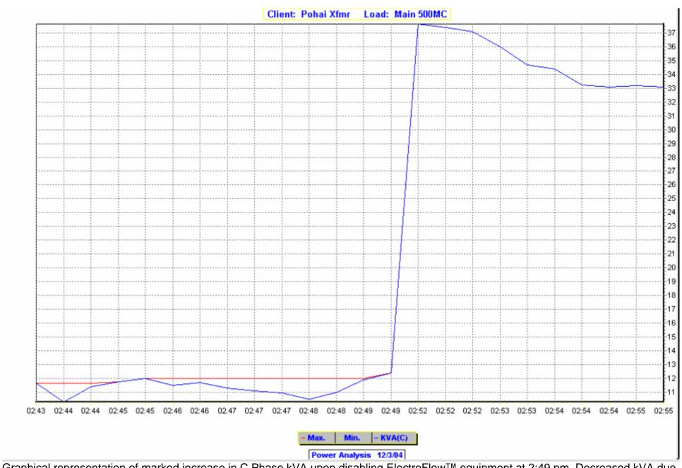
Graphical representation of marked increase in C Phase kVA upon disabling ElectroFlow™ equipment at 2:49 pm. Decreased kVA due to ElectroFlow™ is directly confirmed by HECO billings (typically at page 2.)
